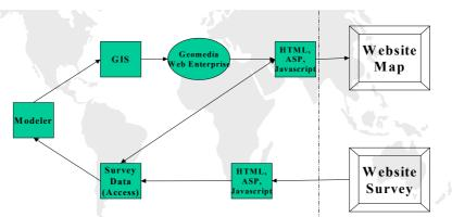
Figure 2: Schematic of OSDSS web implementation
