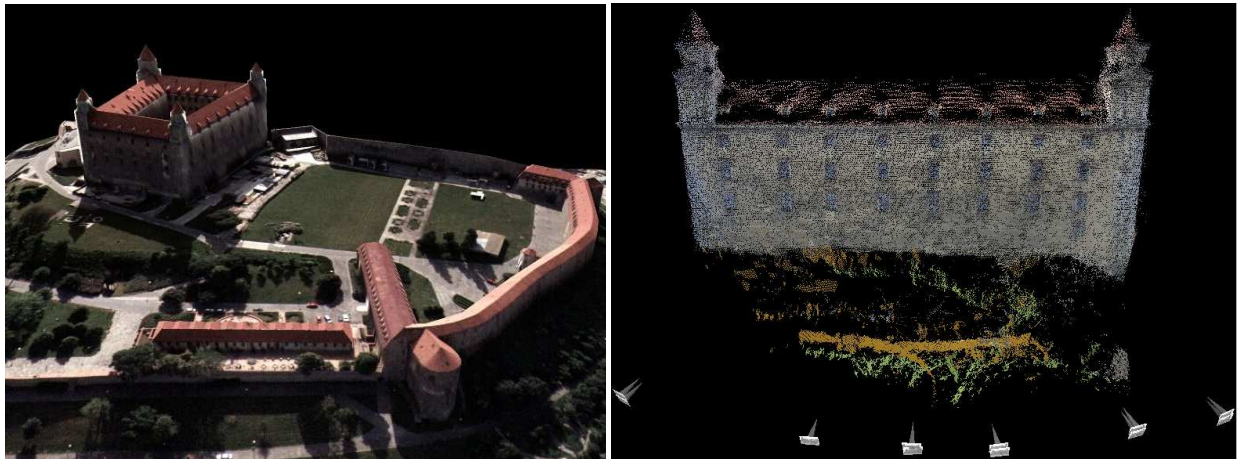
Figure 4: The first 3D urban models: (a) Castle reconstruction with the kind help of Eurosense Slovakia, provided by Peter Borovsky, and (b) the first MetropoGIS reconstructed castle façade by Stanislav Stanek. Input camera positions and the ghosts before their elimination are shown. By the way, the grass area in (a) covered the lost Celtic palace (Carnuntum?).
