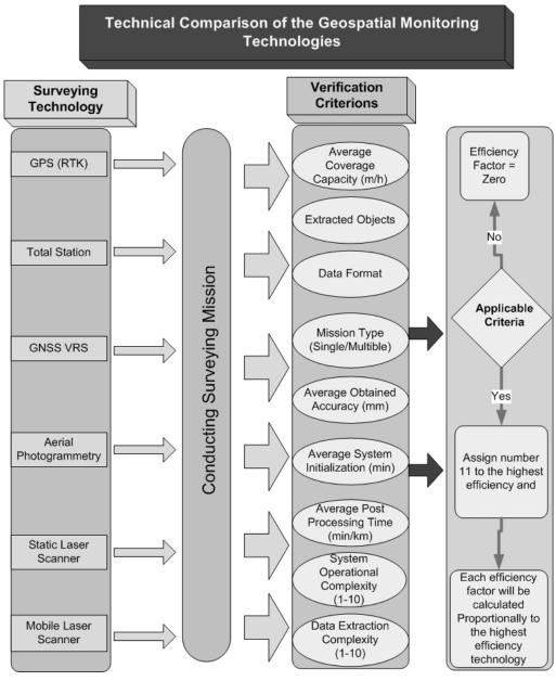
Fig 1: Technical comparison of the geospatial updating technologies.
