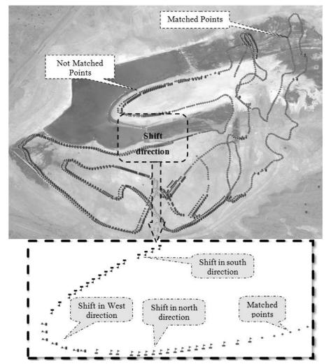
Fig 2: Matched and directions of not matched RTK GPS points with mobile laser scanning GPS.
