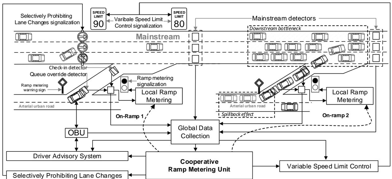
Fig. 1: Illustration of downstream bottleneck location with cooperative ramp metering architecture
