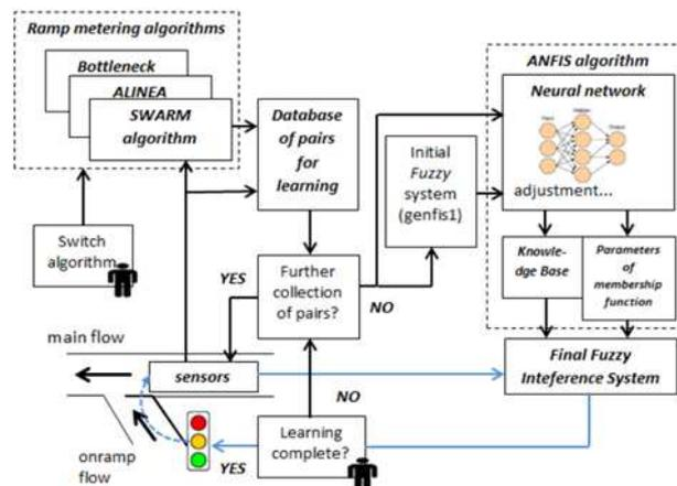
Figure. 2: Scheme of ANFIS algorithm for ramp metering control.
