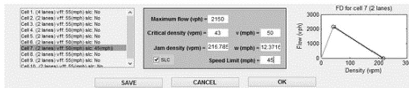
Fig. 5: Fundamental diagram GUI augmentation for definition of the VSLC.
