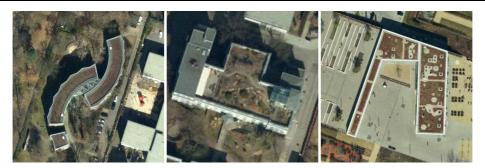
Fig. 3: Greenery: 2a) extensive and 2b) intensive green rooftop, 2c) biodiversity.
