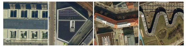
Fig. 6: Solar energy: 4a) semi-transparent photovoltaics, 4b) and 4d) photovoltaics and solarthermics, 4c) glass greenhouse.
